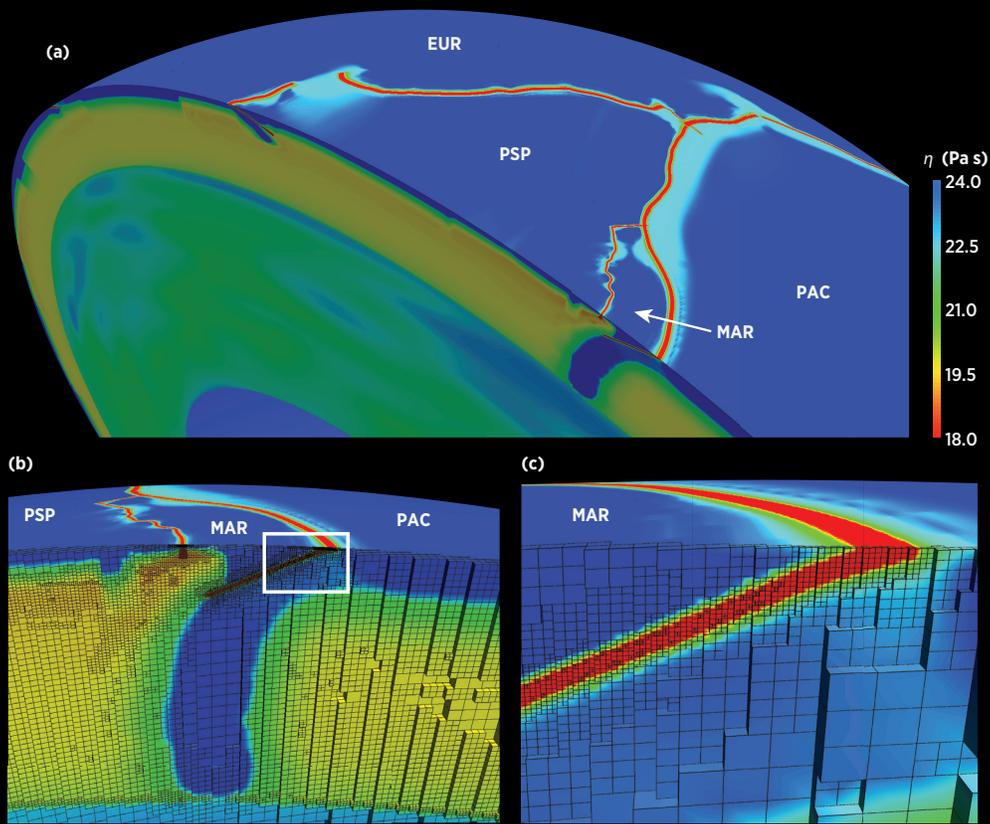
(a) Cutout showing viscosity in a global mantle flow model through the Marianas and Philippines. (b) Zoom-in on viscosity of the Marianas subduction zone, showing the mesh. (c) Further zoom-in on the hinge of the Marianas slab, as denoted by the white box in (b). Plate labels are: **EUR**: Eurasia; **MAR**: Marianas; **PAC**: Pacific; **PSP**: Philippine Sea (from Alisic et al, 2012).
